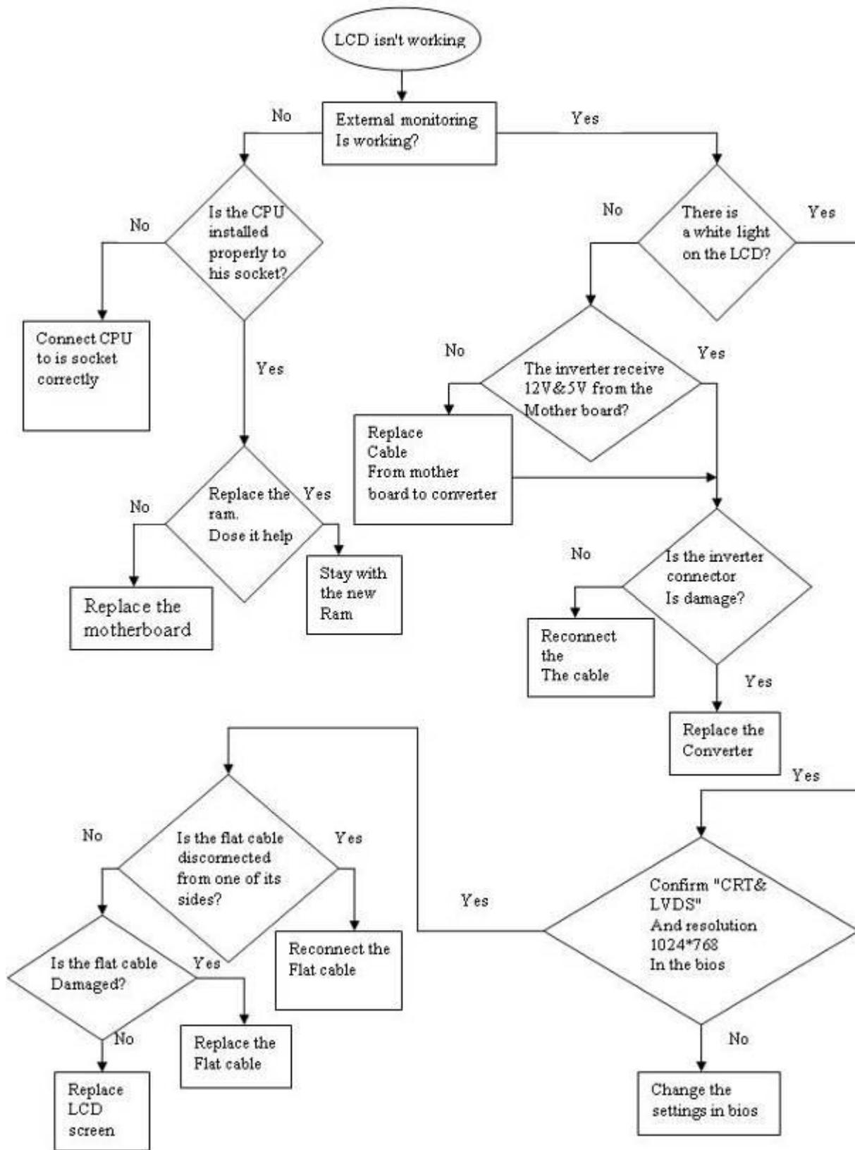
Figure 17-3 Block Diagram LCD
