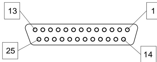
Figure 15-1 Analog channels connector pin out
