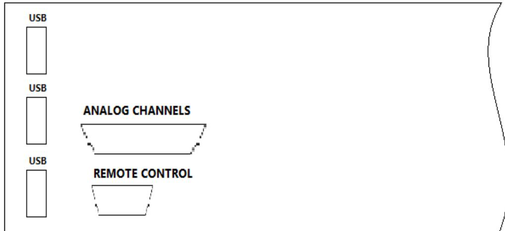
The DIGI-LITE™ system comes complete with all software loaded. If no damage was incurred during shipping, it is necessary to attach all the components to the main console. Figure 4-1 shows the back panel with all connectors.
